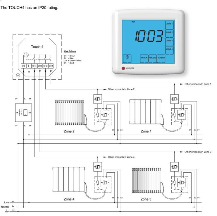
PLEASE NOTE: THE TOUCH4 IS A PROGRAMMER ONLY. TO CONTROL THE TEMPERATURE OF THE ELECTRIC DÉCOR AND COLUMN RADIATORS, THE SUPPLIED RF THERMOSTAT MUST BE USED. PLEASE REFER TO THE ELECTRIC DÉCOR, ELECTRIC COLUMN AND TOUCH4 INSTALLATION INSTRUCTIONS FOR MORE INFORMATION
