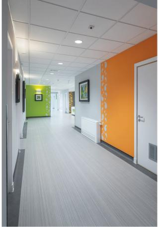
MYSON's range of LST radiators were chosen due to the high quality and reputation of the brand and being compliant with NHS Estates Guidance notes 1998 which means they are ideal for hospital and care home applications. The radiator's surface temperature is designed to remain below 43°C and are built with a safety conscious round steel casing, eliminating sharp edges and emitting any safety concerns.
