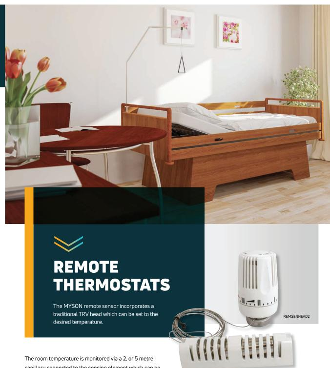
The room temperature is monitored via a 2, or 5 metre capillary connected to the sensing element which can be mounted in a convenient and temperature representative area of the room. Remote sensor heads are ideal for use when it is difficult for a traditional TRV to operate, such as behind furniture or in direct sunlight, and are primarily used with LST radiators.
